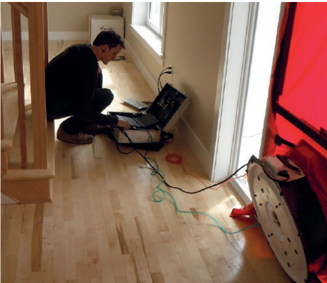
A blower door test measures the air exchange rate in a home, a key component in testing the air-tightness of the structure and contributes to determining a home's EnerGuide rating.
