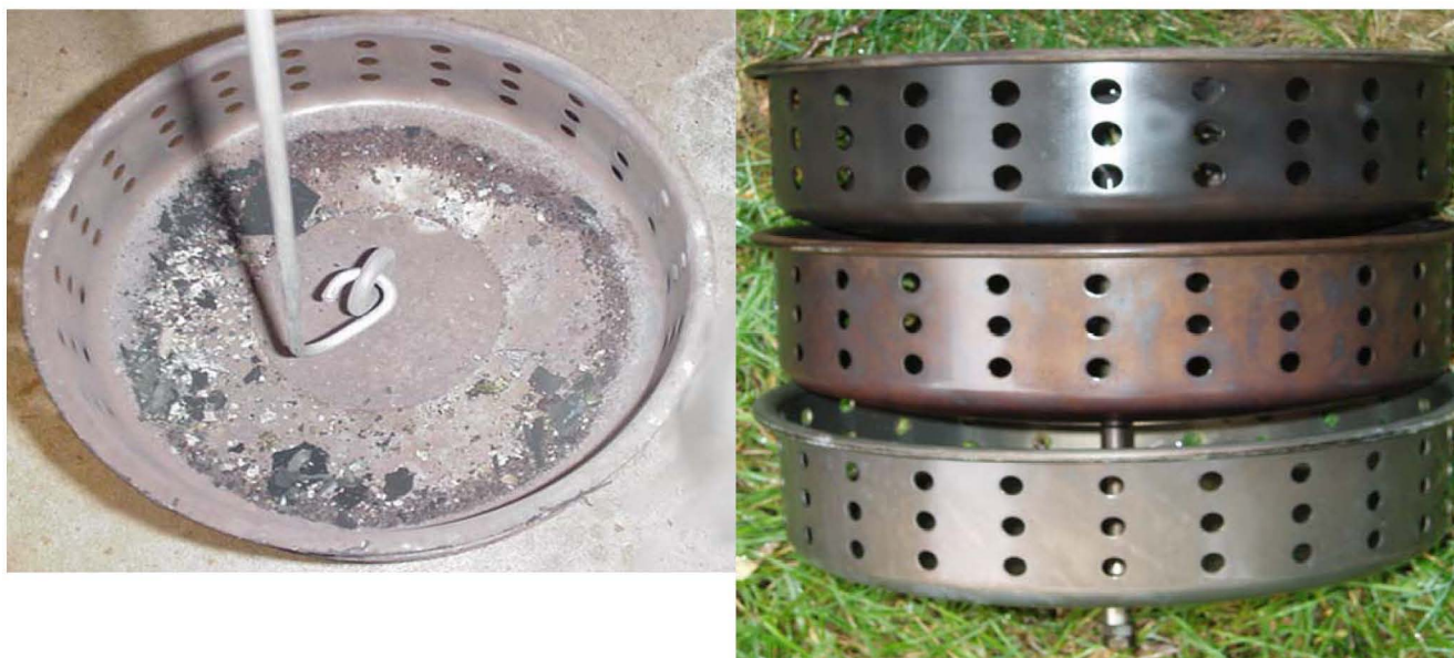
Figure 25 Upper "jet" before (left) and after cleaning
