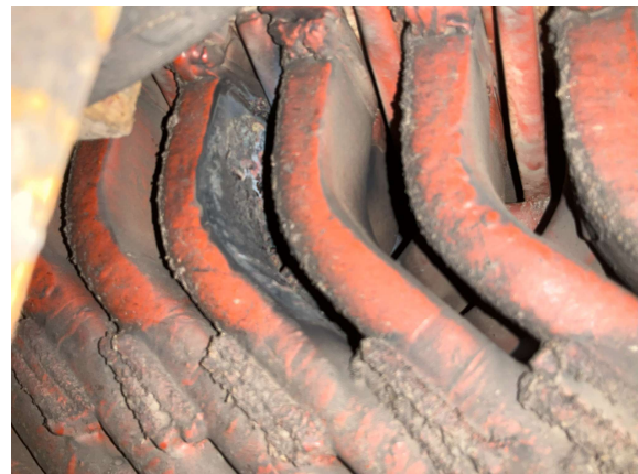
Above picture showing one of the coils which had failed.
