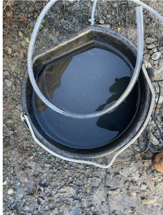
Photo 3: Observed mineral oil sheen in groundwater from monitoring well MW5. Photo taken on December 12, 2024.
