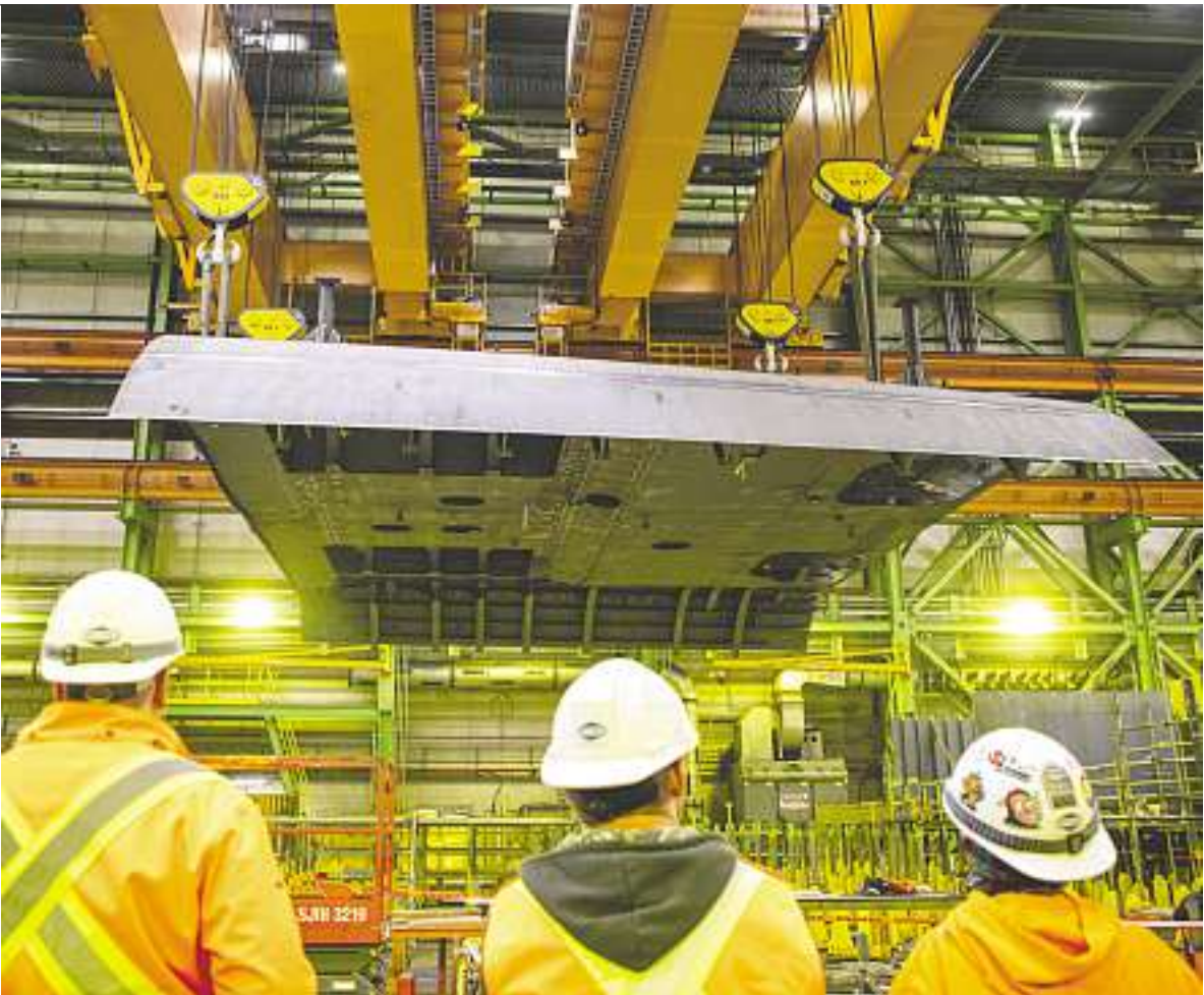
The first hull component of a River-class destroyer is lifted at Irving Shipyard in Halifax.
