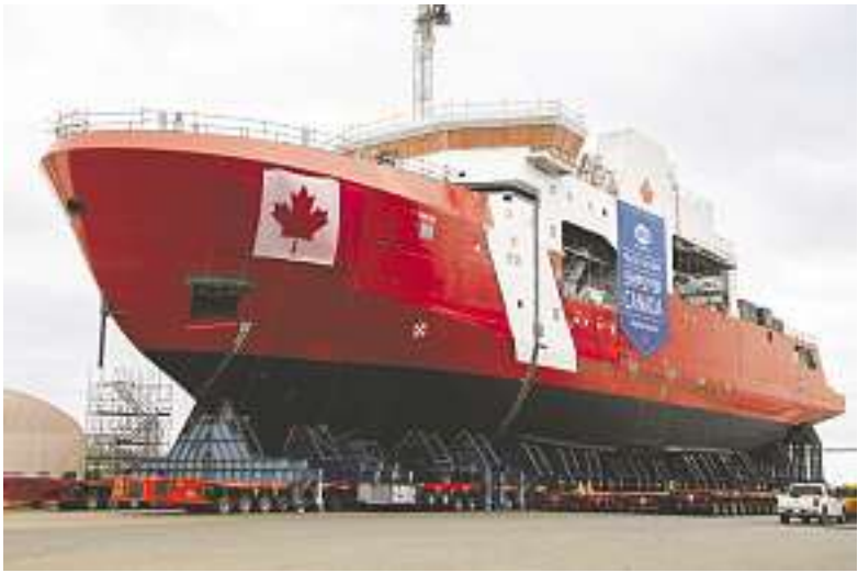
An Arctic and offshore patrol ship built for the Canadian Coast Guard nears completion at the Irving Shipyard in Halifax.
