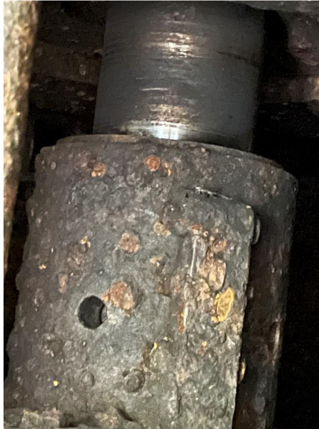
Figure 26: Runner shaft scoring
