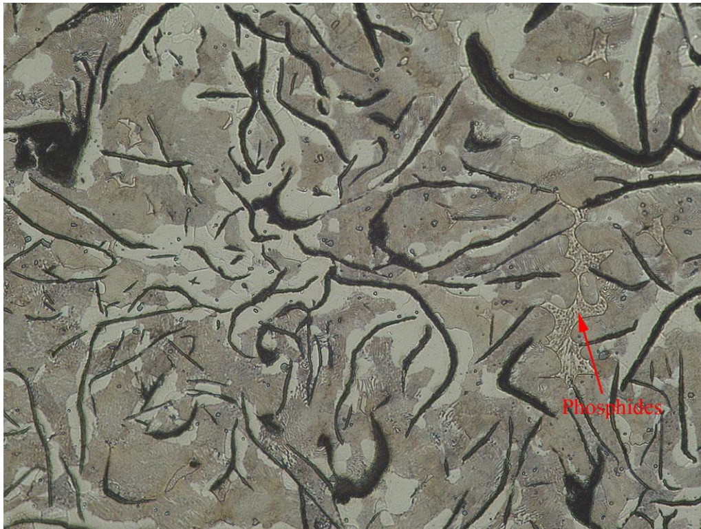
Figure 6 O2 T etched microstructure showing pearlite, phosphides 500x
