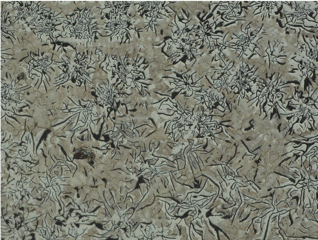
Figure 4 O2 L Unetched microstructure showing rosette formations near outside 200x.jpg
