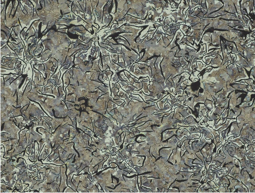
Figure 3 O1 L etched microstructure showing rosettes 200X
