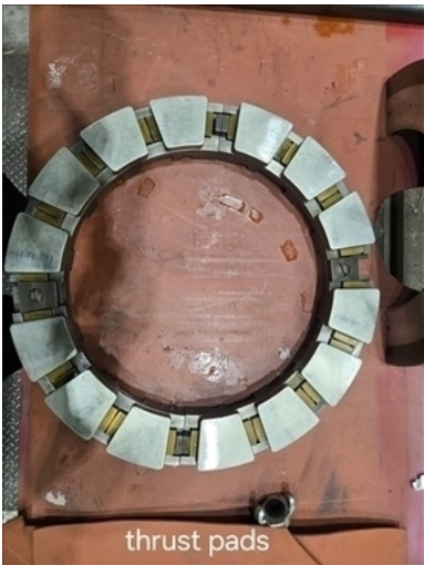
2.4.1.5 Bearing #2 Thrust Pads
