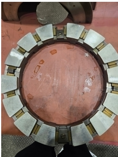
2.4.1.6 Bearing #2 Thrust Pads
