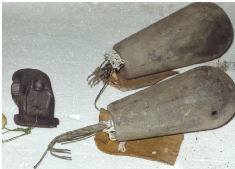
Figure 17 Low frequency Stockbridge damper with messenger wires fatigued due to galloping. (Havard Engineering In. Archive)
