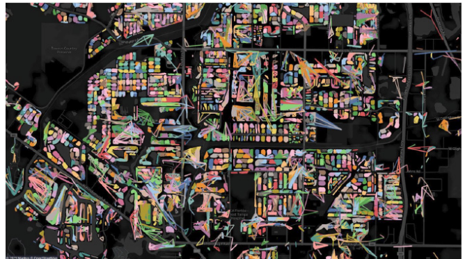
Location Awareness: Meter-to-Transformer Visualization of Groupings
